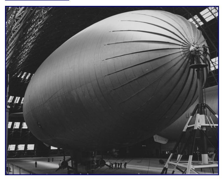
ZP-11 ZNP-K type blimp being inspected inside NAS South Weymouth's LTA Hangar One.on May 2<sup>nd</sup> 1944 after suffering what was characterized as "envelope abrasion". If you look carefully, you can see the abrasion marks on the bottom half of the blimp's gasbag behind the nose stiffening battens
